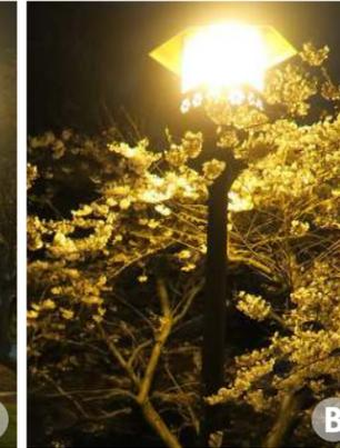
Correlated Color Temperature (CCT)\* of light sources throughout the neighborhood is typically 3500K in the case of the current pedestrian pole light, 4000K for roadway lights, and 2200K for High Pressure Sodium floodlights. As such, the variety of sources create a patchwork experience of lighting color at night. (A)
